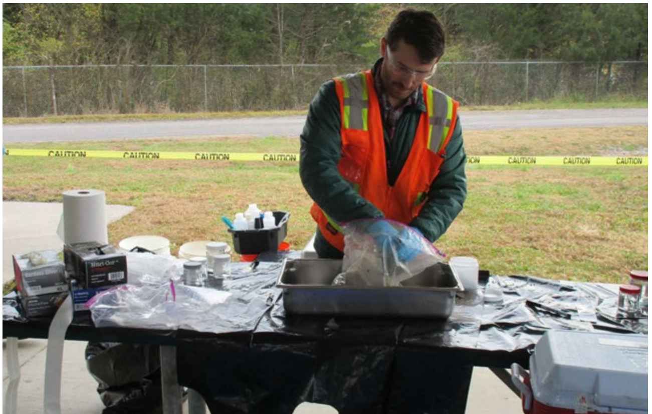
Photo 5. CEC Compositing the 5 subsamples or aliquots for each mixed sample. (Source: TDH, December 1, 2021).
