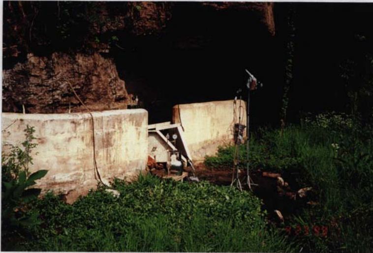
Photograph No. 1 Facing northwest: Ambient air sampling at Wilson Spring. Sampling Station A-7. Sampling heights – 3 & 5 feet above ground surface.
