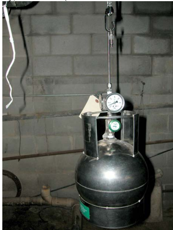
FIGURE 3 - Photo of the SUMMA canister setup, Concord Cleaners, 3706 Hillsboro Pike. Nashville, Davidson County, Tennessee. (Photo credit: David Borowski, TDH, 1/19/05)
