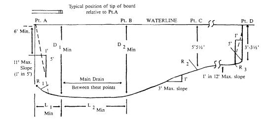
NOTE: Placement of boards shall observe the following minimum dimensions. With multiple board installations minimum pool widths must be increased accordingly.
