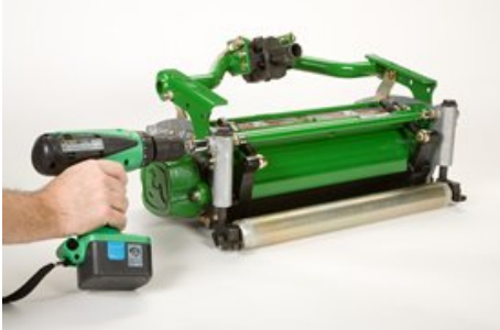
Adjustment with cordless drill
