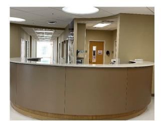
As can be seen by the attached pictures, the nurse's station is a rounded countertop with a desk area inside. The plexiglass wall section must be installed at the outer edge of the countertop to prevent anyone from being able to jump on and/or stand on the countertop. The plexiglass shall be a minimum of 0.25" thick or thicker depending on the type of
