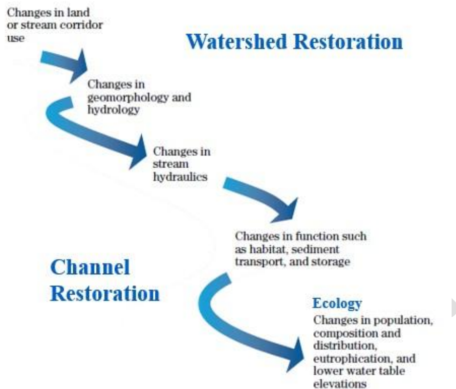
Figure 3.2. Example watershed disturbance resulting in a causal chain of alterations to stream corridor structure and function ( from NRCS 2007).
