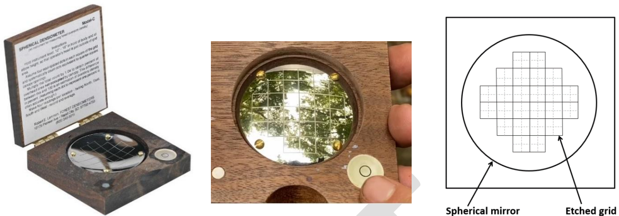
Figure 6.20. Photo of a US Forest Service densiometer, photo of grid cells with tree canopy on the mirror, and illustration of subdivided boxes for each data collection point (Cook et al. 1995).
