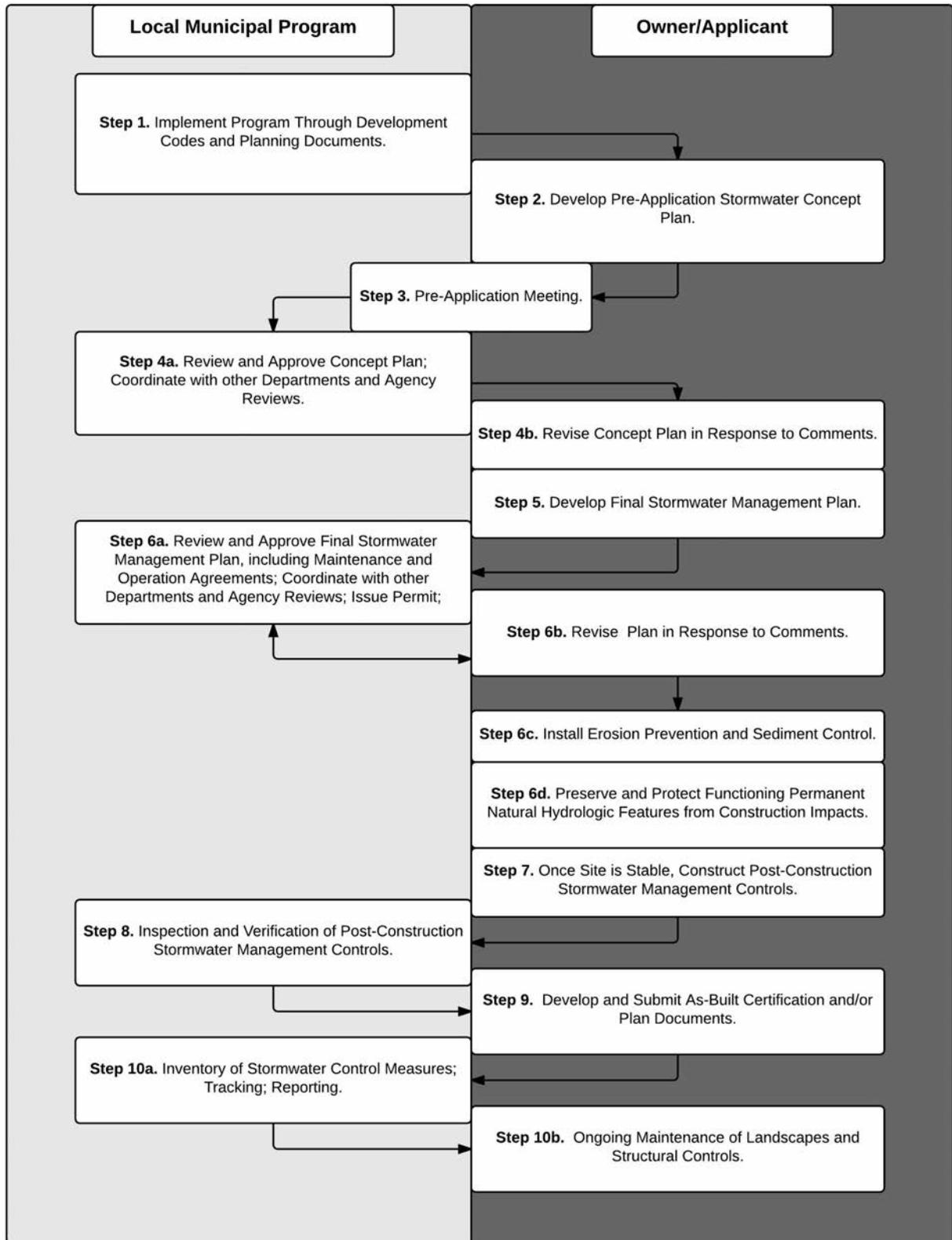
Figure 2.5: Typical Compliance Pathway for Permanent Stormwater Runoff Management for New Development and Redevelopment Projects.
