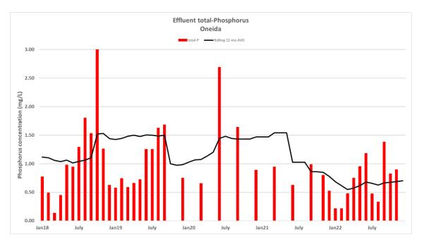
Oneida staff found that there is an optimal amount of mixing for phosphorus removal. Too much mixing and the sludge blanket doesn't become septic enough. Too little mixing and the sludge blanket becomes too septic. During winter months, one of two submersible mixers operating at a
