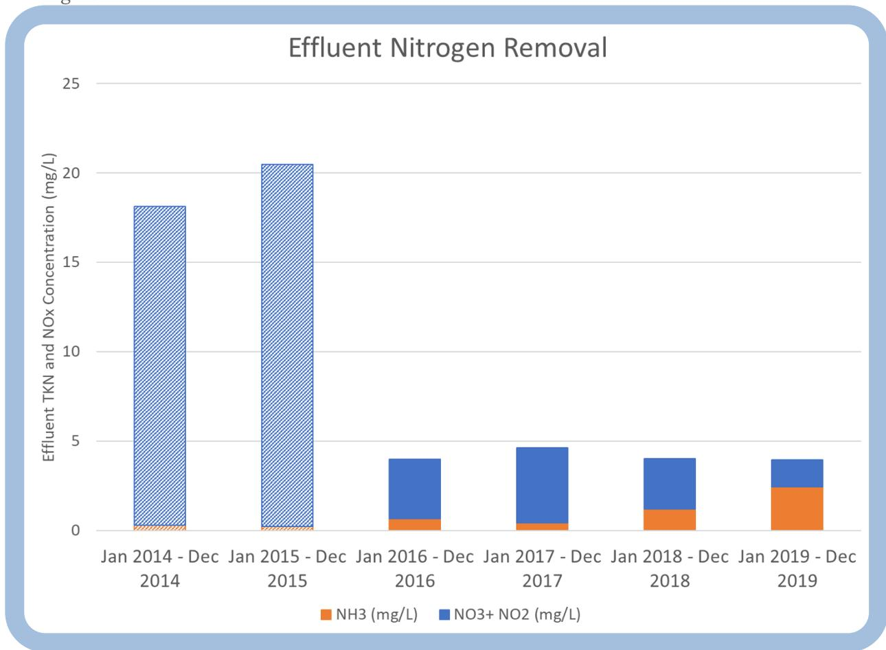
6. Average effluent total nitrogen (mg/L) from baseline (Jan 2014 – Dec 2015) and Jan 2016 – Dec 2019
