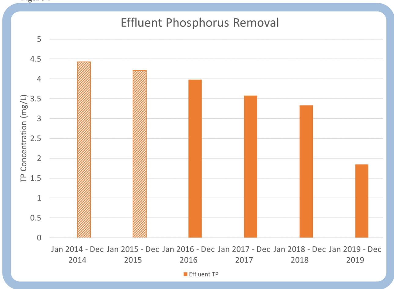
5. Average effluent total phosphorus (mg/L) from baseline (Jan 2014 – Dec 2015) and Jan 2016 – Dec 2019
