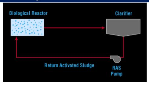
**Bio-Tiger Model - Biokinetic Model that Simulates Activated Sludge Processes**
