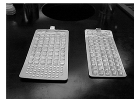
Left: The 97 well QuantiTray 2000 will count up to 2419 cfu without dilution. Right: The 51 well QuantiTray will count up to 200 cfu without dilution.
