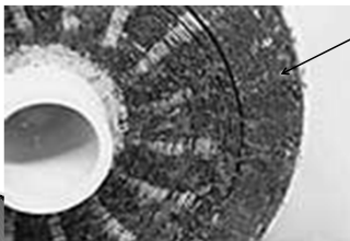
Extreme biofouling of membrane.
