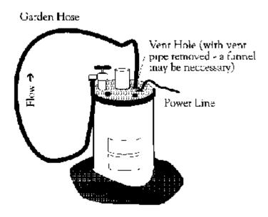
Pump water through all outlets in the plumbing by opening faucets until water smells of chlorine. If it does not, add more chlorine bleach to the well. Shut the power off to the well system and remove the garden hose from the system and recap the well. Turn the power back on to the pumping system.
