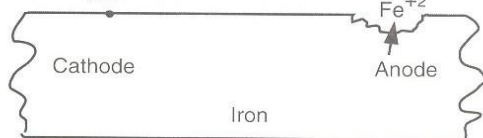
D. Rust forms
