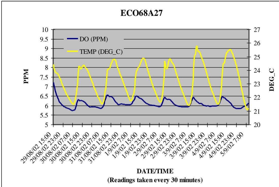
**Figure 10: Diurnal dissolved oxygen and temperature data, Island Creek reference site, Cumberland Plateau (68a). Readings every 30 minutes for 162 hours.**
