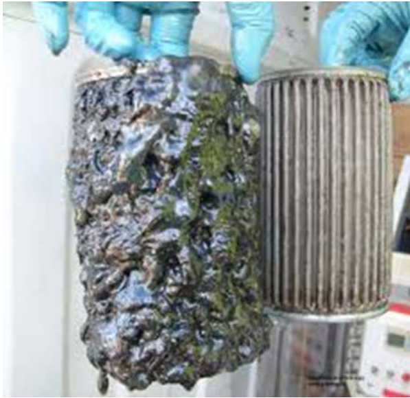
Figure 3: Microbial plugged dispenser filter compared to a filter with no microbial contamination 7
