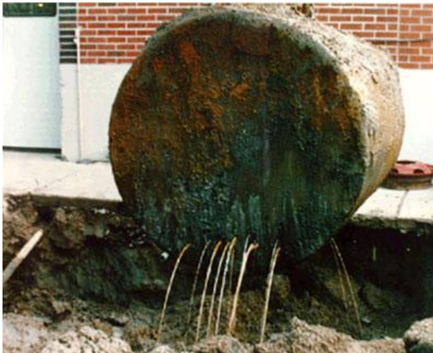
*Without proper corrosion protection, you may have a release.*
