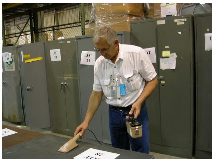
John Wojtowicz scans a surplus desk to verify that DOE is following proper radiological control procedures (TDEC photo)
