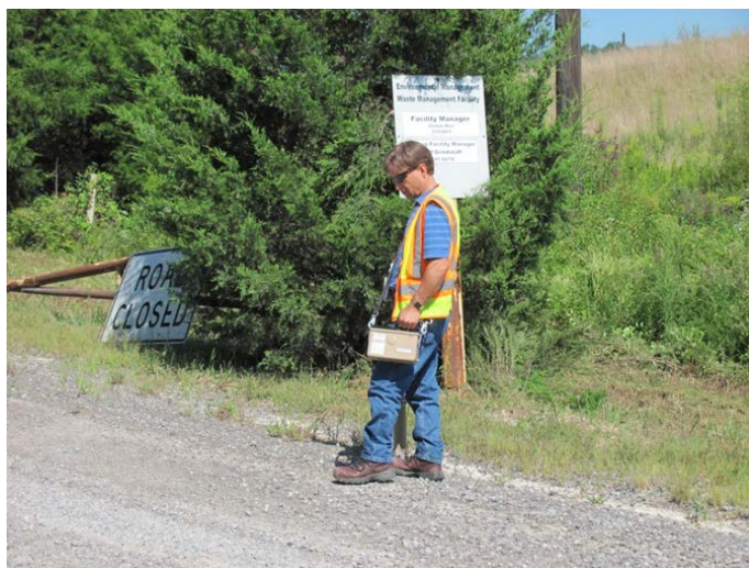
David Foster conducts a radiological survey of the EMWMF haul road. (TDEC photo)
