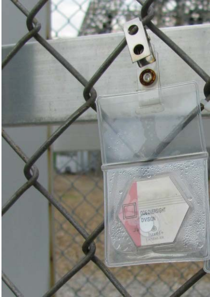
Environmental Dosimeter used to monitor quarterly dose at each location
