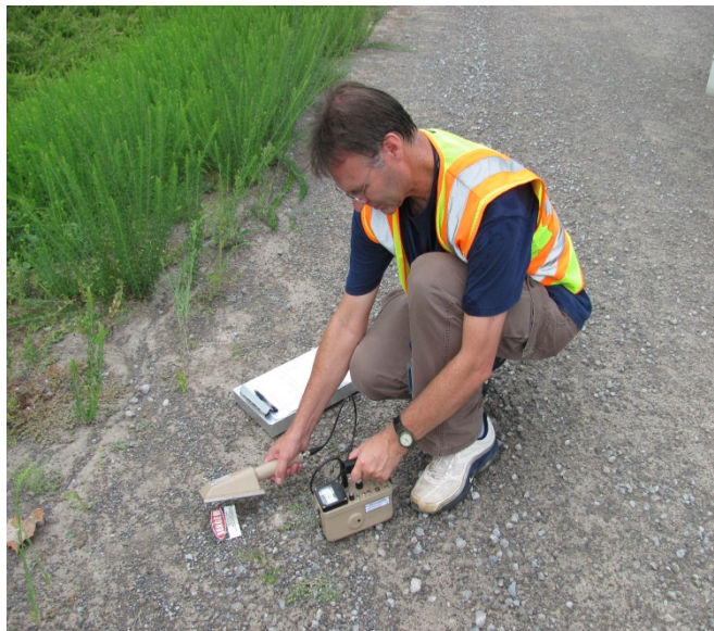
Robert Storms scans an item found on the Haul Road for alpha/beta/gamma contamination.
