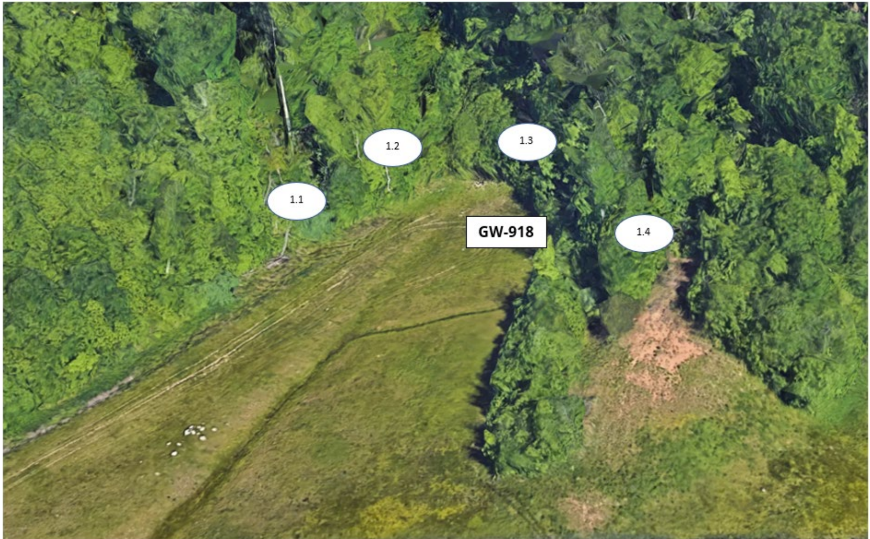
Figure 5.1.3: Sample Location 1. The four locations were composited and identified as sample EMW-PROAD01
