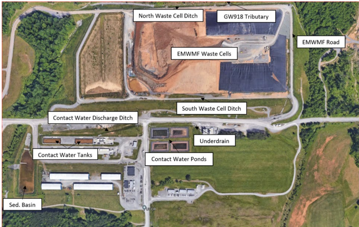
Figure 5.1.1. Map of EMWMF north and south waste cells drainage ditch locations.
