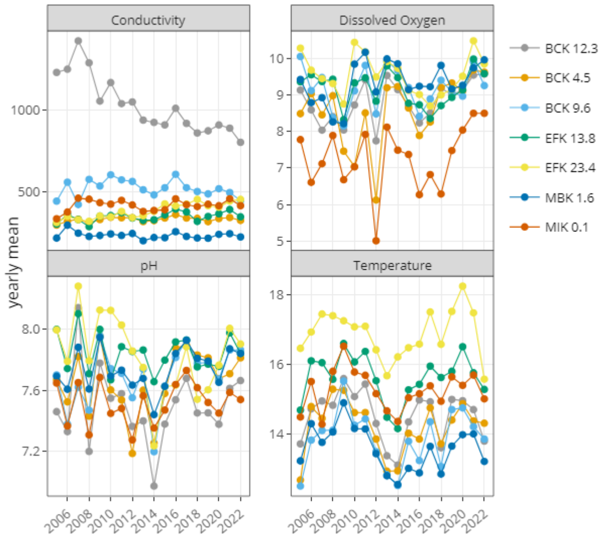
Figure 8.1.3: Mean annual values for Conductivity, Dissolved Oxygen, pH, and Temperature from 2005 to the present for all sites. Units for conductivity, dissolved oxygen, pH, and temperature are \mu\text{S/cm} , mg/L, std. unit, and ^{\circ}\text{C} , respectively
