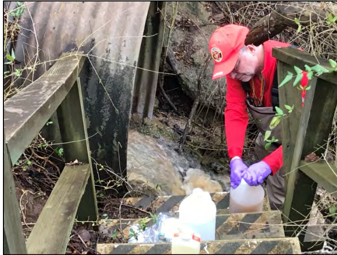
Figure 5.3.2: TDEC Staff Collecting Samples Following a Rain Event (Photo was taken by Mike Coffey, CDMSmith.)
