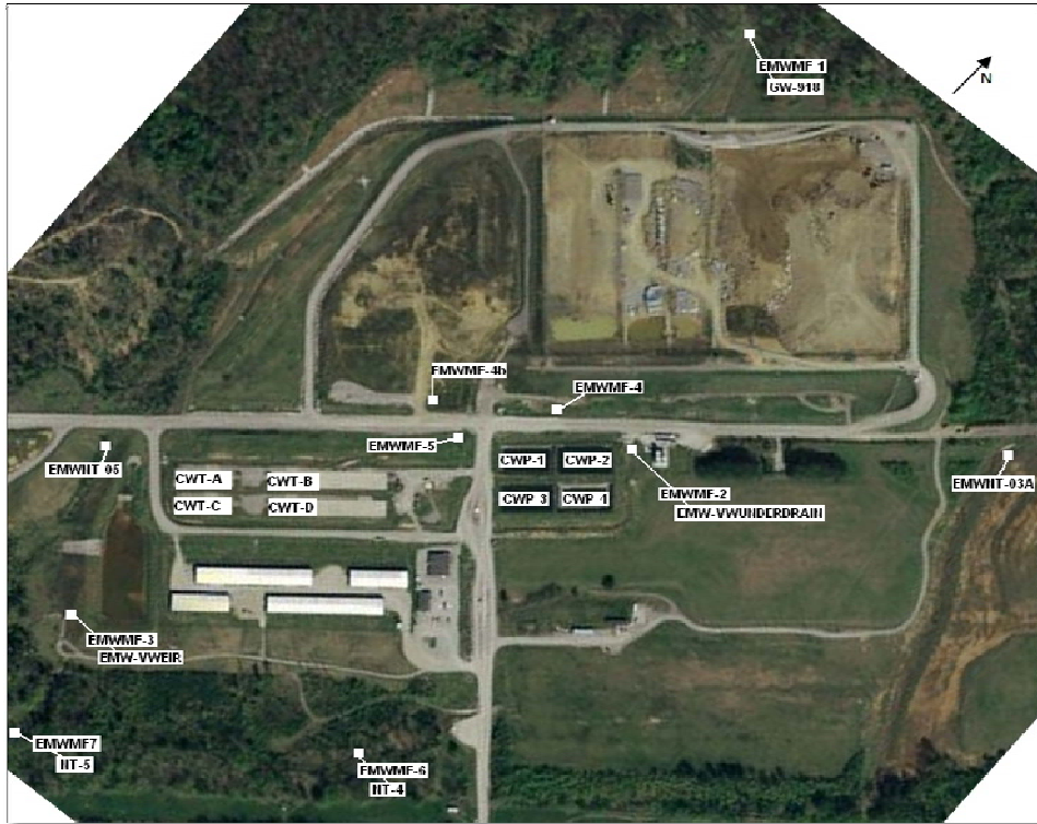
Figure 1: Surface Water / Groundwater / Contact Water Sample Locations at EMWMF DigitalGlobe, GeoEye, US Geological Survey, USDA Farm Service Agency (2010) Google Maps [online]
