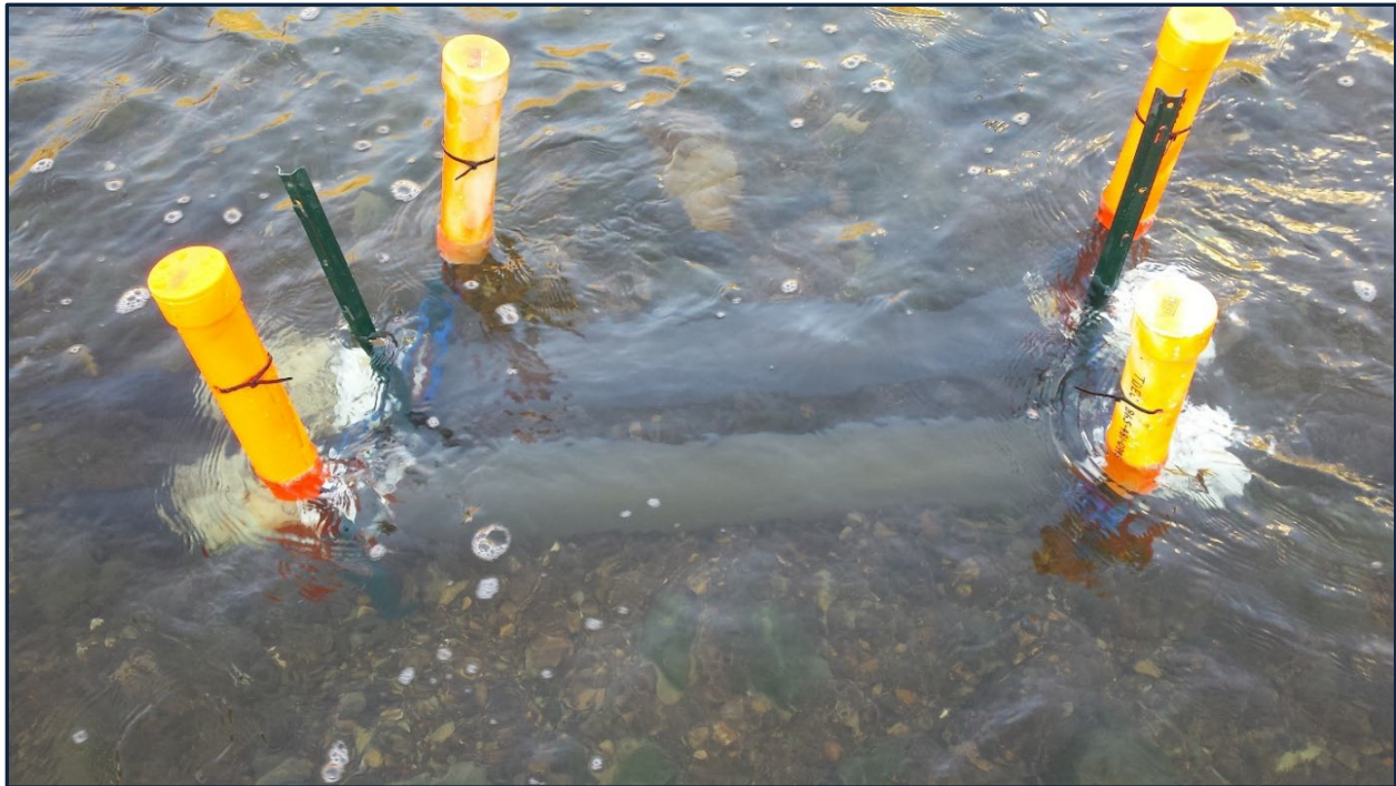
Figure 8.1.8.2: Tandem sediment trap installation in East Fork Poplar Creek
