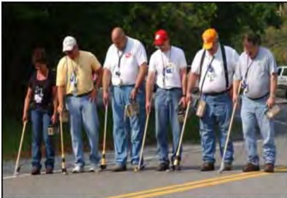
Radiation survey on Hwy. 95 after liquid waste leaked during transit (DOE/ORO-2183, Type B Accident Investigation Board Report).
