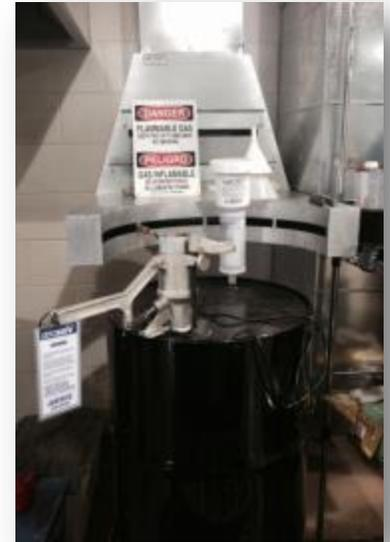
Picture 4: Aerosol puncture system with vent
