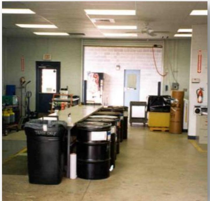
Picture 2: Proper drum segregation and labeling.
