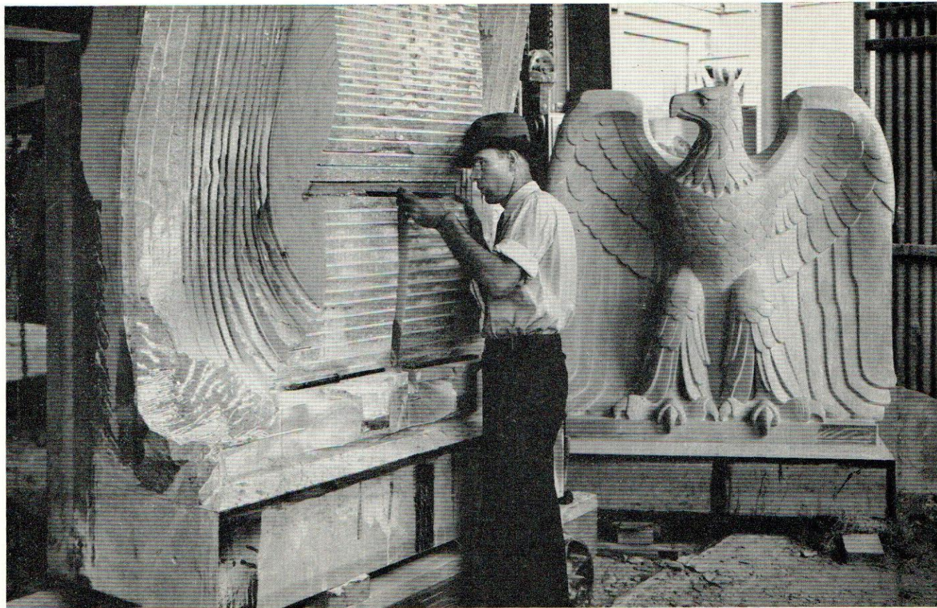
FIGURE 5. Craftsman producing eagle figure from marble. (Photo courtesy Ty-Sa-Man Machine Co., Knoxville)
