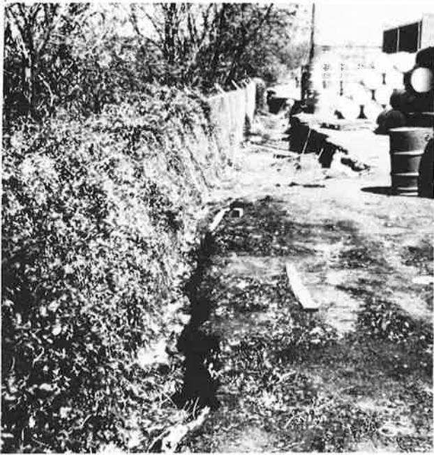
Figure 1. Large slump on alluvium located (Environmental Map Index No. 17) 1,000 ft. (305 m) west of Cameron Hill.
