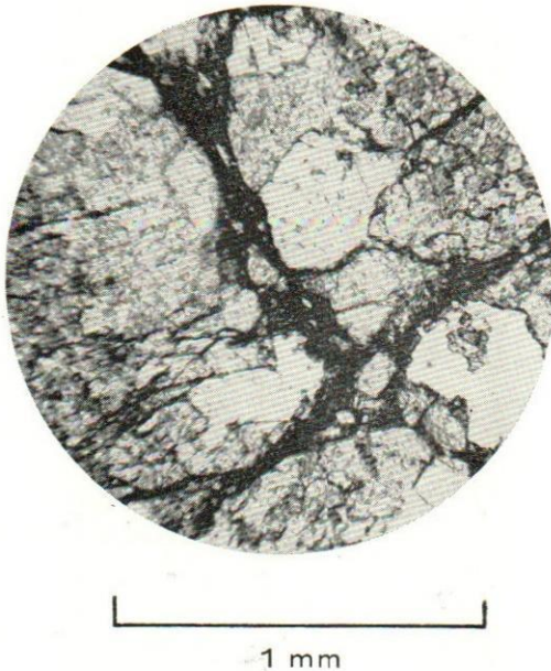
FIGURE 51.—Thin section (plane polarized light) of crackle breccia in Knox Dolomite. Sample is from deep drill hole on Central Hill. Recrystallization of dolomite along fracture margins is indicated by large grains. These have been fractured by a later stage of deformation.
