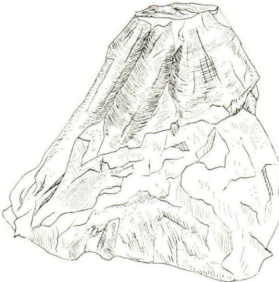
FIGURE 36.—Blast cone showing sharp ridges and rounded concave valleys (drawing by R. A. Miller). Specimen is about 4 inches wide at the base.
