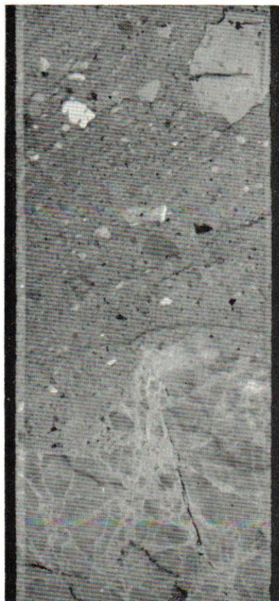
FIGURE 57.—Core sample from deep drill hole showing relationship of crackle and heterogeneous rubble breccias. Note that fractures of crackle breccia terminate abruptly at contact with rubble breccia, which suggests that crackle breccia is earlier. Also note bedding lineation (or flow banding). Core diameter is about 2 inches.
