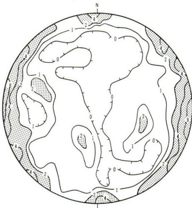
FIGURE 29.—Preferred orientation diagram showing the fabric of 309 poles to bedding in the outcrop area of Knox and Stones River Groups, mainly in the central megabreccia zone in Wells Creek Basin.
