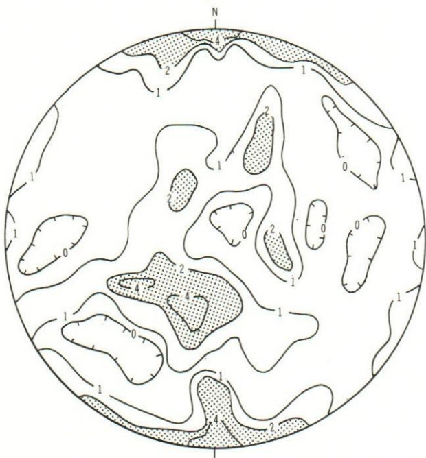
FIGURE 30.—Preferred orientation diagram showing the fabric of 328 poles to bedding in the Ordovician, Silurian, and Devonian rocks outside the megabreccia zone in Wells Creek Basin.
