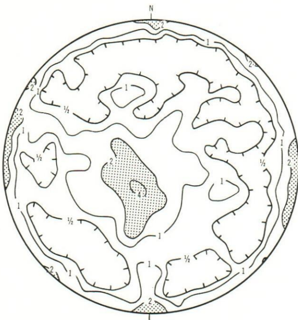
FIGURE 28.—Preferred orientation diagram showing the fabric of 1027 poles to bedding in all parts of the Wells Creek structure. Contours on this figure and figures 29, 30, and 31 are percent of poles that fall within 1 percent of the area of the net, as is standard for contouring such plots.
