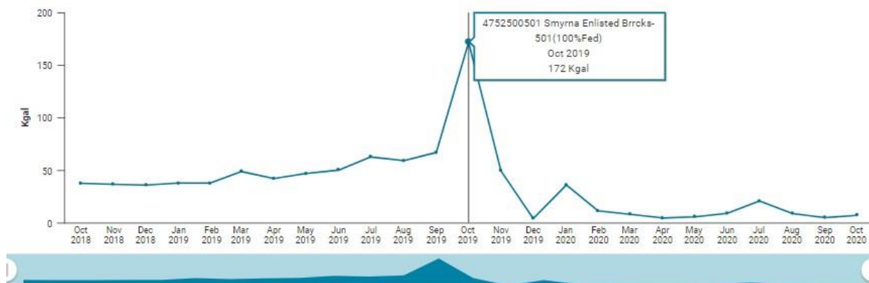
[A.3] Figure 6.3.1b – Department of Military October 2019 Water Usage with Water Leak (UDM Dashboard)
