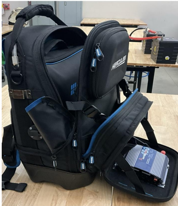
2nd Prototype: Solar Backpack Steel cables added excessive weight to the tool backpack, even with the switch to a lighter lithium battery.
