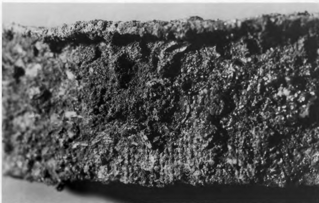
Figure 84. Textile pseudomorph adhering to a tinware container rim (84-85-10I2).
