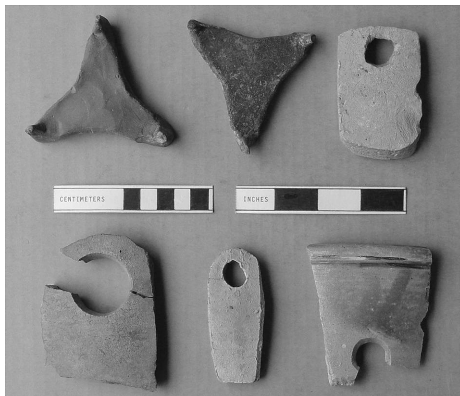
Figure 1-19. Kiln furniture items, D (three-pointed stilts and draw tiles).
