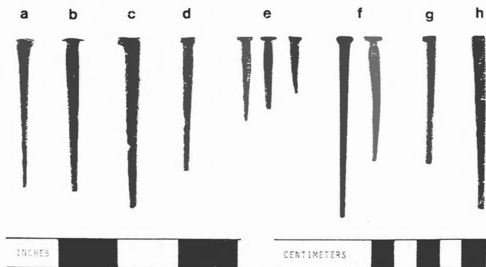
Figure 57. Early machine-cut nails: hand headed - (a) rose head, (b) T-head, (c) L-head, (d) square head; machine headed - (e) lath nails, (f) common nails, (g) L-headed, (h) headless.
