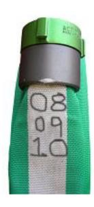
15. Booster hose shall be tested to 250 psi for 5 minutes.
