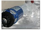
Mid-Matic fog nozzle) provides the air aspiration needed for a good blanket. When the nozzle is set in the *straight stream* position, less air is aspirated into the solution resulting in a thinner blanket of foam, but allowing a farther reach. Conversely, when the fog nozzle is set to the *fog* position, less distance is achieved, but a thicker blanket of finished foam is produced.
