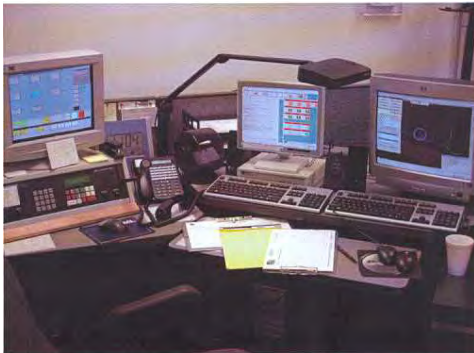
Console Layout (l to r) – Radio, CPE, Map Display
