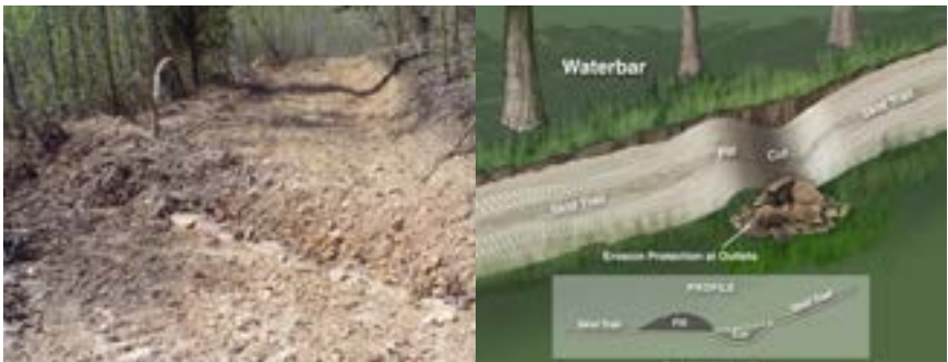
Figure 7a. Water bar construction
