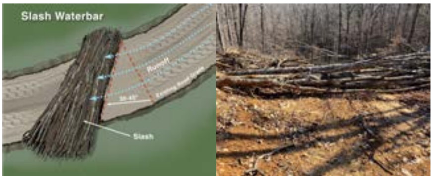
Figure 7b. Water bar construction
