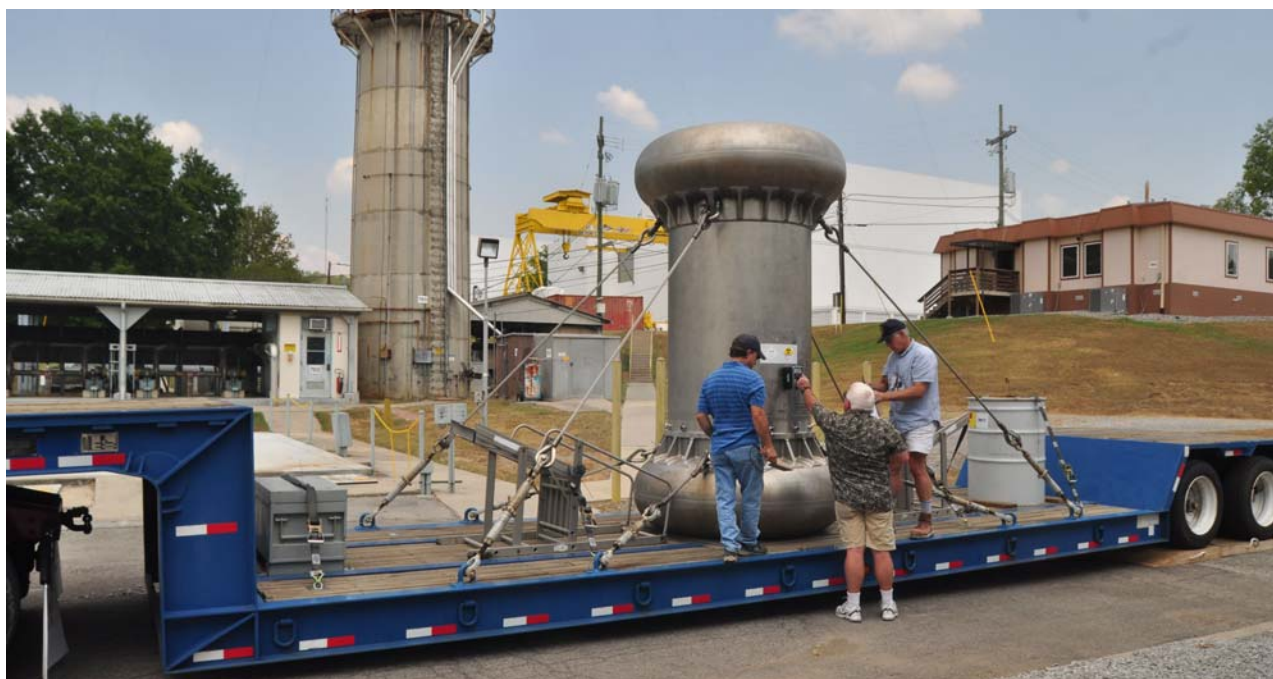
David Foster (left) and John Wojtowicz (right) are taking readings with Ludlum alpha/beta radiation detection devices on the surface of the cask. Phillip Roush , Natalie Pheasant , and Dave Thomasson assist in the inspections when needed. The cask pictured is a specially designed, shielded cask used specifically for transporting Spent Nuclear Fuel.
