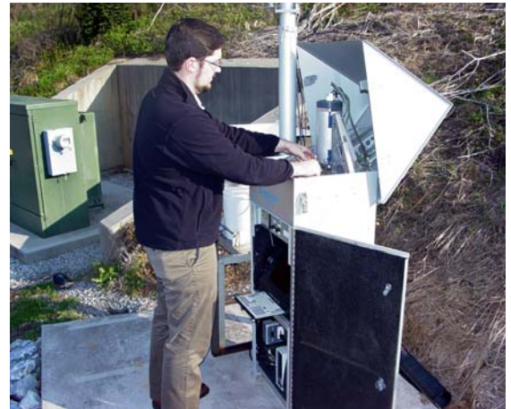
DRH Health Physicist Daniel Sims conducting air and rainwater sampling using the RadNet sampling unit during the Japanese incident.
