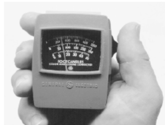
Fig. 1 Footcandle meter. The meter is used to measure “illuminance.” It is the only measuring instrument that you need for most applied lighting efficiency work. Being an older model, this meter indicates in units of footcandles. Newer models indicate in units of lux.
